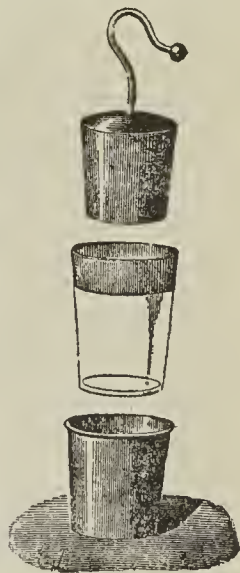
FIG. 11 Modern form of Leyden jar with movable coat- ings
